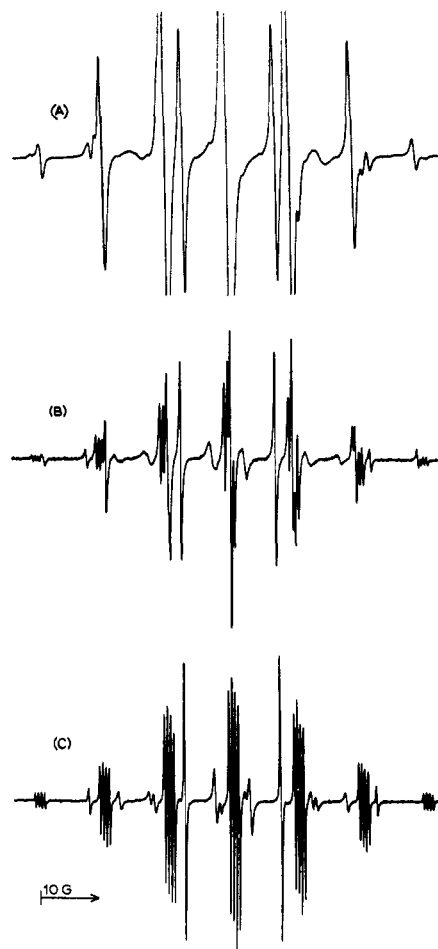
Figure 5. Effect of time on the products observed in the reduction of perfluorobiacetyl with lithium metal in THF, (A) immediately after reduction. The cis species is mainly 2c, the trans species is in the fast exchange mode, (B) after 10 min at 25°; 2a is now clearly seen; the trans species is in the slow exchange mode; (C) after 30 min there is no longer any evidence for 1c or 2c. The spectrum no longer changes with time.
