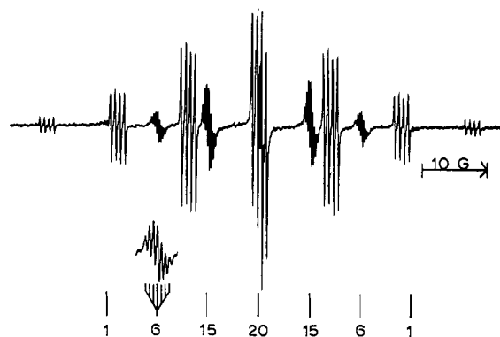
Figure 7. Reduction of perfluorobiacetyl by lithium in isopropyl ether. A mixture of 2a and 1c (with hfs by 2\text{Li}^+ ) is observed at 25°.
